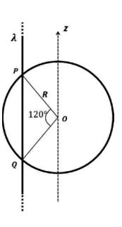
Further electric field is perpendicular to the wire therefore its z-component will be zero.
